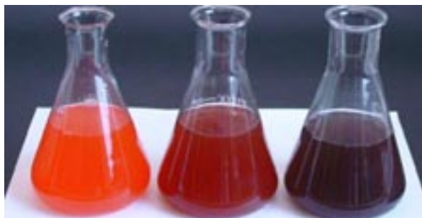
Figure 4 Analysis of Vitamin C in red capsicum (pepper). Left flask: Before the endpoint the solution retains its original colour. Centre flask: Once all the ascorbic acid has been oxidised, a slight excess of added iodate produces a dark starch-iodine complex, giving the solution a purple colour. This is the titration endpoint. Right flask: If a further mL or two of iodate were to be added after the endpoint, the solution would develop the dark purple colour shown here.
