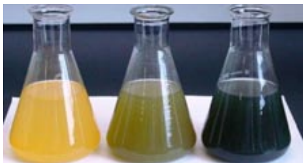
Figure 3 Analysis of Vitamin C in freshly squeezed orange juice. Left flask: before the endpoint, the colour of the solution reflects the bright orange colour of fresh orange juice. Centre flask: Once all the ascorbic acid has been oxidised, a slight excess of added iodate forms a starch-iodine complex, a green colour in this case. This is the endpoint of the titration. Right flask: If further iodate solution were to be added after the endpoint..
