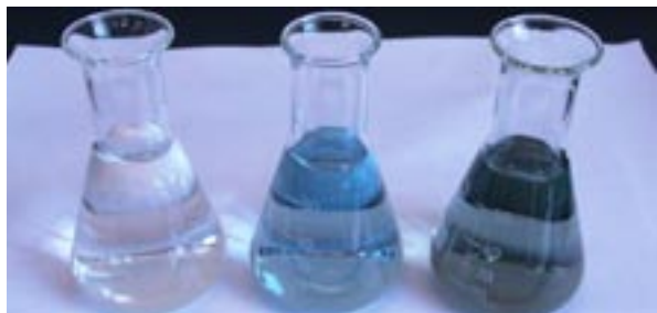
Figure 1 Titration of a colour-free Vitamin C tablet. Left flask: before endpoint, iodine formed from added iodate reacts with ascorbic acid leaving the solution colourless. Centre flask: At the titration endpoint all the ascorbic acid has reacted and the slight excess of added iodate reacts to give a pale blue colour due to starch indicator. Right flask: If addition of iodate is continued after the endpoint, further starch-iodine complex is formed, giving the solution a stronger blue-black colour..
