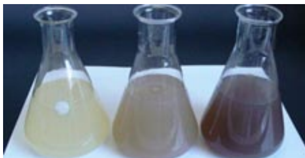
Figure 2 Analysis of Vitamin C in a commercial fruit juice. Left flask: before the endpoint. This colour is initially unaffected by the addition of iodate, as the resulting iodine reacts with ascorbic acid present. Centre flask: At the titration endpoint any excess iodate added reacts to produce a dark starch-iodine complex. In this case from yellow to brown-grey. Right flask: This flask is shown to illustrate the effect of adding just a mL or two more of iodate solution after the endpoint is reached.
