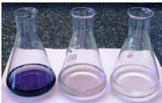
Figure 3. A series of flasks showing the colour change as the last remaining iodine (with added starch indicator) is titrated with thiosulfate. The dark blue-black colour disappears, leaving a colourless solution at the endpoint.
