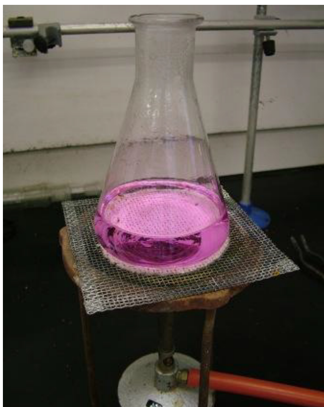
Figures 1 – 4. Development of purple colour due to formation of \text{MnO}_4^- in steel sample solution. Figure 1 shows the nearly colourless solution containing dissolved steel, before any oxidation of manganese has occurred. As the solution is heated over a period of about 20 minutes the purple colour of \text{MnO}_4^- gradually becomes stronger and stronger, as shown in Figures 2, 3 and 4.
