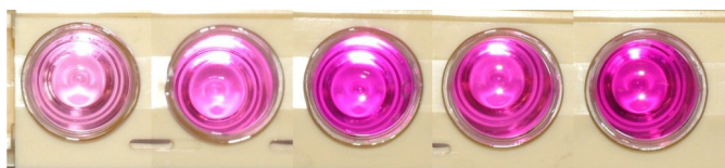
Figure 6. The same boiling tubes as in Figure 5 ( \text{MnO}_4^- standard solutions with concentrations of 0.5 - 2.5 \times 10^{-4} \text{ mol L}^{-1} ) viewed from above, looking directly down the length of the tube. This view provides the most accurate "eyeball" comparison of the solutions' colour intensities.
