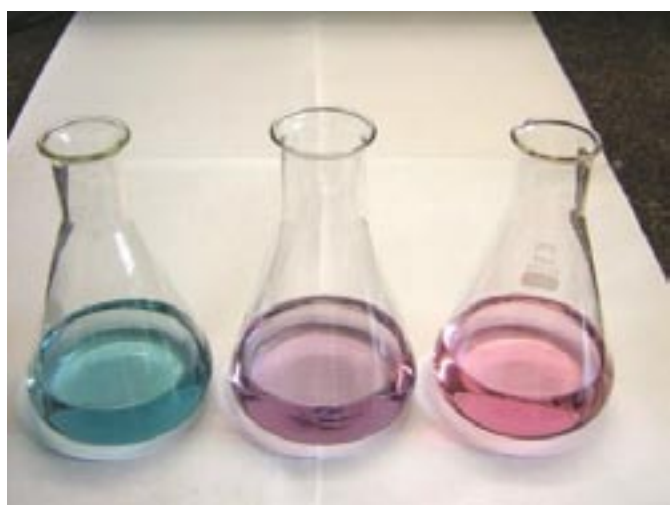
Figure 1 Colour changes for magnesium chloride back-titration in clear solution using Eriochrome Black T indicator. Left flask: blue colour well before endpoint (all \text{Ca}^{2+}/\text{Mg}^{2+} ions complexed by excess EDTA, all indicator molecules uncomplexed). Centre flask: last trace of blue/purple colour just before endpoint (excess EDTA almost totally complexed by added \text{Mg}^{2+} ). Right flask: pink/red colour at endpoint (all EDTA complexed by added \text{Mg}^{2+} , indicator also complexed).
