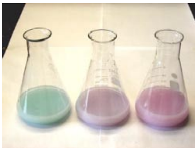
Figure 2 Same colour changes for magnesium chloride back-titration as in Figure 1, but for cloudy (opaque) sample solution, eg milk. Left flask: blue colour well before endpoint. Centre flask: last trace of blue/purple colour just before endpoint. Right flask: pink/red colour at endpoint.
