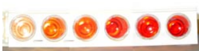
Figure 5. The same boiling tubes as in Figure 4 (prepared using \text{Fe}^{3+} standard solutions with concentrations of 2 - 12 \times 10^{-5} \text{ mol L}^{-1} ) viewed from above, looking directly down the length of the tube. This view provides the most accurate “eyeball” comparison of the solutions’ colour intensities.
