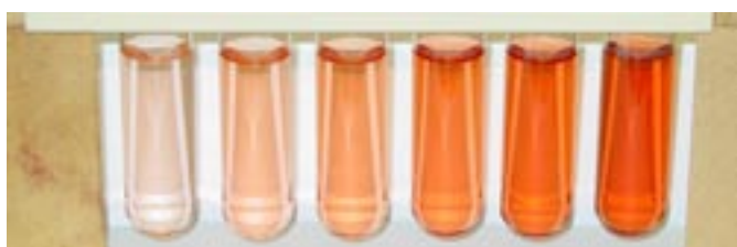
Figure 4. Blood-red coloured solutions produced by the ferric thiocyanate complex ion ( \text{Fe}[\text{SCN}]_2^+ ). These solutions were prepared using the following range of \text{Fe}^{3+} standards: 2, 4, 6, 8, 10, 12 \times 10^{-5} \text{ mol L}^{-1} .
