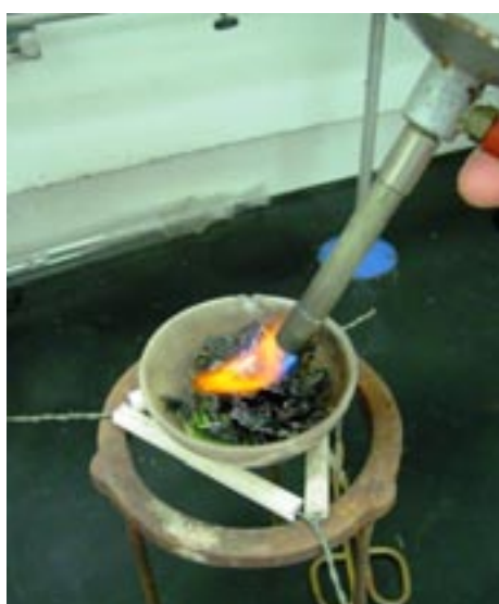
Figure 2. Set up used for combusting a silverbeet sample directly in the bunsen burner flame.
