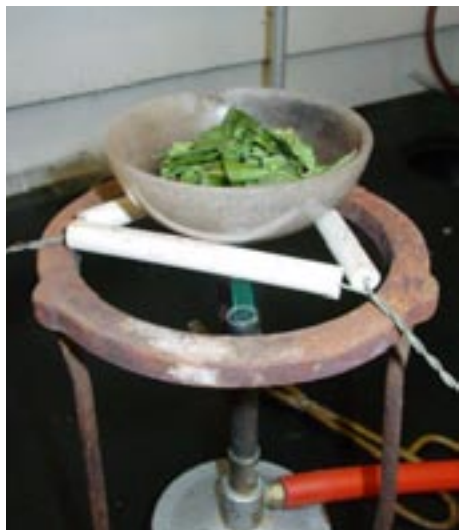
Figure 1. Set up used for heating a silverbeet sample in a crucible.
