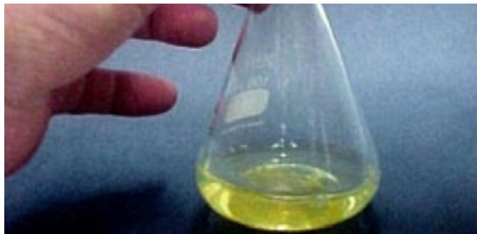
Figure 1 Before the addition of any silver nitrate the chromate indicator gives the clear solution a lemon-yellow colour.
