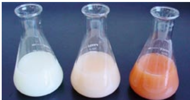
Figure 2 Left flask: before the titration endpoint, addition of Ag + ions leads to formation of silver chloride precipitate, making the solution cloudy. The chromate indicator gives a faint lemon-yellow colour. Centre flask: at the endpoint, all the Cl - ions have precipitated. The slightest excess of Ag + precipitates with the chromate indicator giving a slight red-brown colouration. Right flask: If addition of Ag + is continued past the endpoint, further silver chromate precipitate is formed
